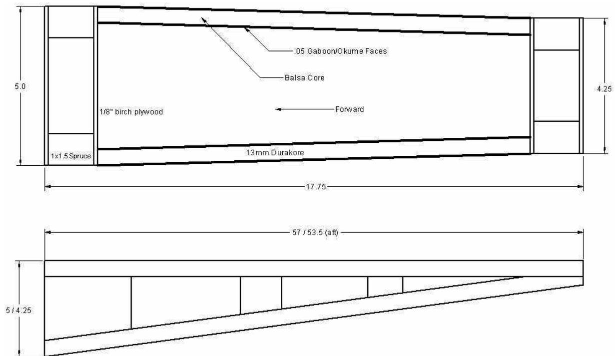
Figure 7 Bugatti Horizontal Stabilizer Spar Detail, with spacer blocks
