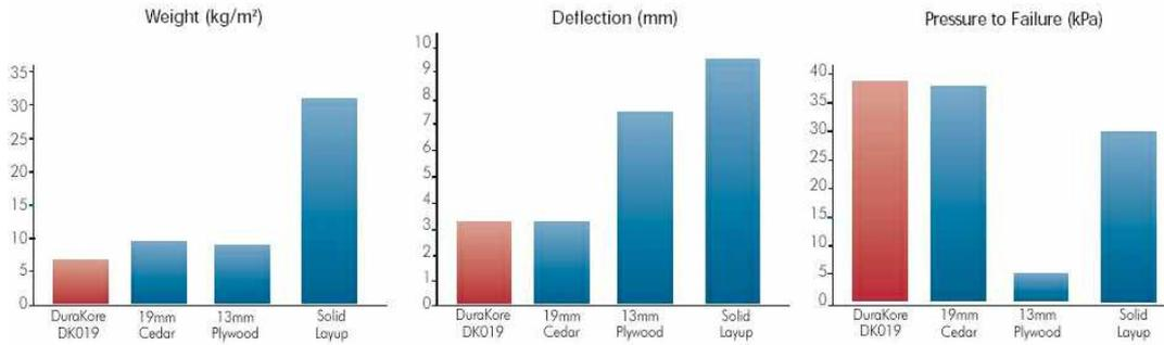
Figure 2 Durakore Material properties (Source: www.atlcomposites.com.au)
