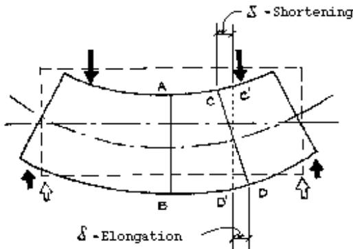
Figure 8 Bending of a beam
