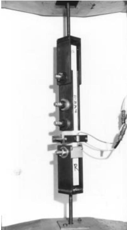
**Figure 2—Test setup for tension parallel-to-grain connection tests.**
