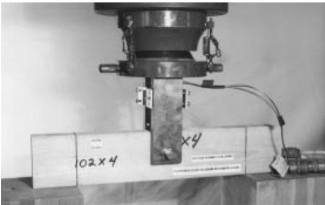
**Figure 3—Test setup for compression perpendicular-to-grain connection tests.**
